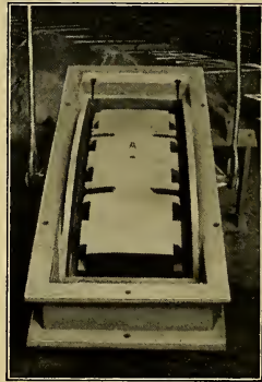
Fig. 11. Tunnel Segment Mould—Lower or Drag Half—Made on a Roll-Over Jolt Machine. In the view shown above, the machine is rolling over the mould after it has been jolted and bottom board clamped.
